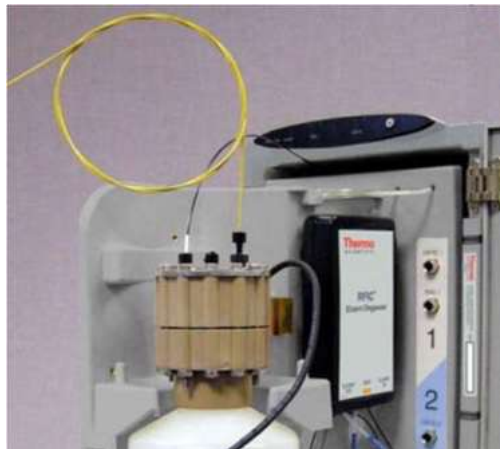
รูปที่ 10-25 Dionex EGC Outlet Connection for Cartridge Conditioning (Standard-Pressure Analytical Cartridge Shown)
